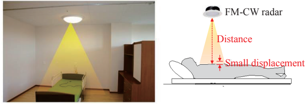
Fig. 3. An example of FM-CW Radar for detecting human breathing
